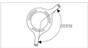
Position the p-shaped chain guard bracket and fasten it onto the drive unit with screws.
