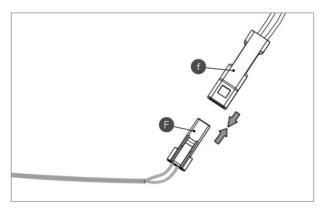
Link the headlight cable to the connector for the headlight at the drive unit.
