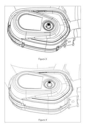
Figures above show how the drive unit looks like when the drive unit cover has been affixed.
