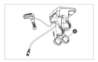
One or two rubber clamping rings may be needed depending on the diameter of the handlebar (the applicable handlebar specifications are Ø22.2, Ø25.4 and Ø31.8). Open the left or right display clamp, and insert one or two clamping rings into the right position of the display clamp as shown in the picture above.
