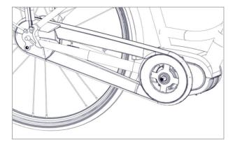
Refer to the chain guard instruction book and install the chain guard after the chain wheel has been installed.
