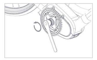
Use a standard tool to fix the lock nut onto the spline shaft.
