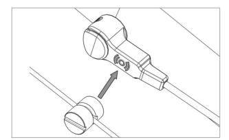
Arrange the speed sensor and the magnet unit as shown in the picture above. When installing the magnet unit, make sure its center is aligned with the center of the speed sensor's induction zone.
