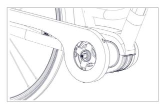
The drawing above shows the mounted p-shaped chain guard.
