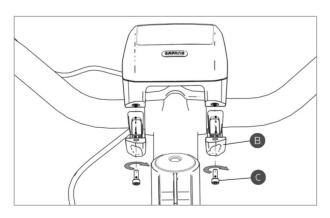
Rubber clamping ring (whose inner diameter is Ø 22.2 or Ø 25.4) 2316020400007 2316020400008 Left and right display clamps for the Ø 22.2 handlebar: Left clamp -2316020400017 Right clamp -2316020400018 Left and right display clamps for the Ø 25.4 handlebar: Left clamp -2316020400007 Right clamp -2316020400008
