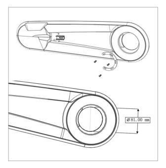
A chain guard binder plate and screws are necessary for installing a full chain guard.
