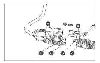
The power bus, which is made up of a positive battery cable, a negative battery cable and battery communication cables, is connected to the battery cables at the drive unit.
